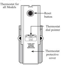
The illustration above shows the temperature adjustment dial used for setting the water temperature. Refer to Operation section of this manual for detailed instructions in how to adjust the thermostat(s).
