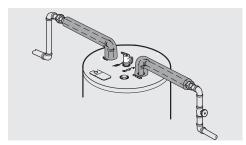
Typical horizontal piping arrangement
