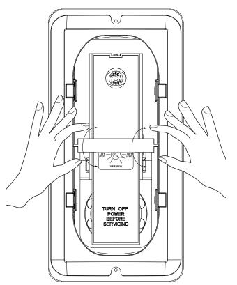
In order to replace the thermostat or heating element, remove the cavity insert crossbar by following the instructions below:
