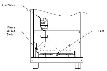
Figure 3: Burner Compartment Area
