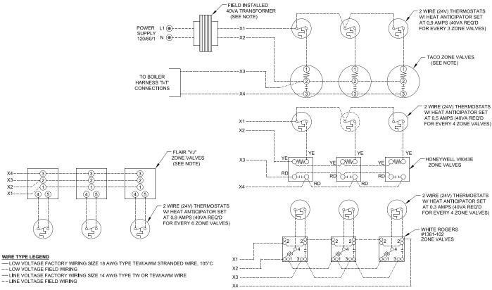
Figure 8-3: Wiring Schematic, Zone Valves
