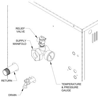
Figure 6-1: Near Boiler Piping
