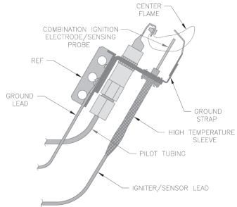
Figure 9-5: Pilot Burner Flame (LP Only)
