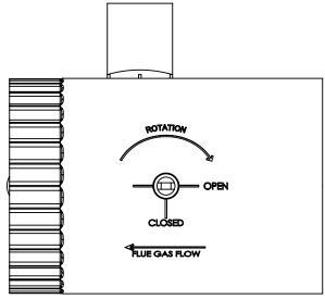
Figure 5-2: Vent Damper Position Indicator
