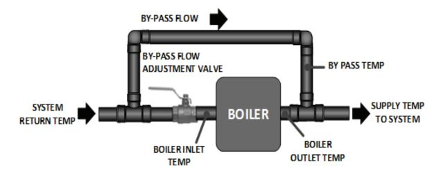
Regardless of by-pass flow, boiler will have inlet temperatures that are same as system return temperature. When boiler inlet temperatures fall below 120°F, boiler will condensate. As by-pass flow is increased, less water flows through boiler which increases boiler temperature rise. This will help reduce propensity for condensation but will not stop it.
