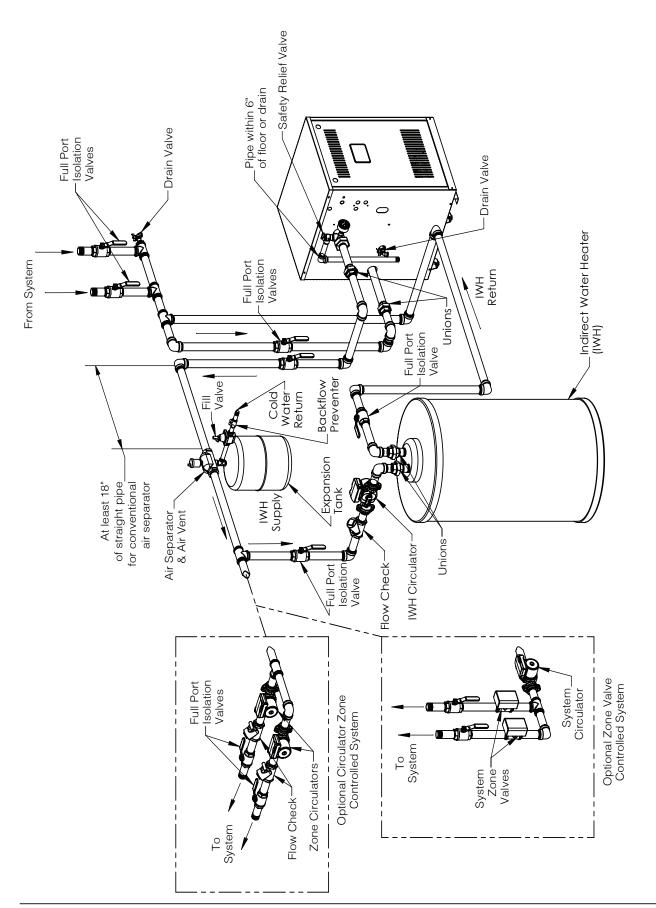
Figure 6-2: Recommended Water Piping for Direct Connection Systems
