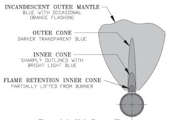
Figure 9-6: Main Burner Flame
