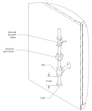
Figure 7-2: Pilot and Gas Piping
