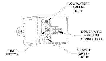
Figure 9-1: IDL 1200 Low Water Cut-Off
