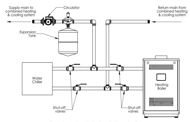
Figure A-1: Isolated Boiler from Refrigeration System
