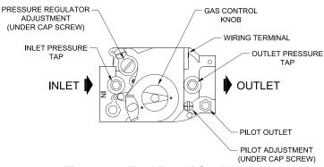
Figure 9-3: Top View of Gas Valves
