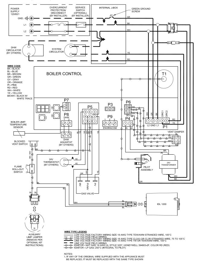
Figure 8-1: Wiring Connection Diagram
