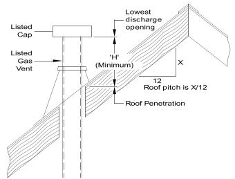
Figure 5-3: Termination Location for Gas Vent
