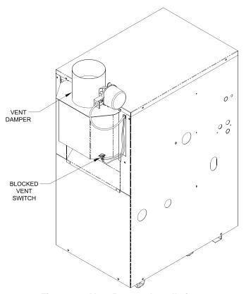
Figure 5-1: Vent Damper Installation
