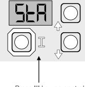
Press "I" key on control to change from one parameter to next. Each setting will alternate between display code and value.
