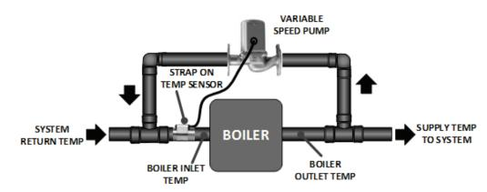
A strap on temperature sensor measures boiler inlet temperatures. This temperature signal is sent to a variable speed pump that will ensure boiler inlet temperatures are always greater than the factory by-pass kit set point of 120°F.
