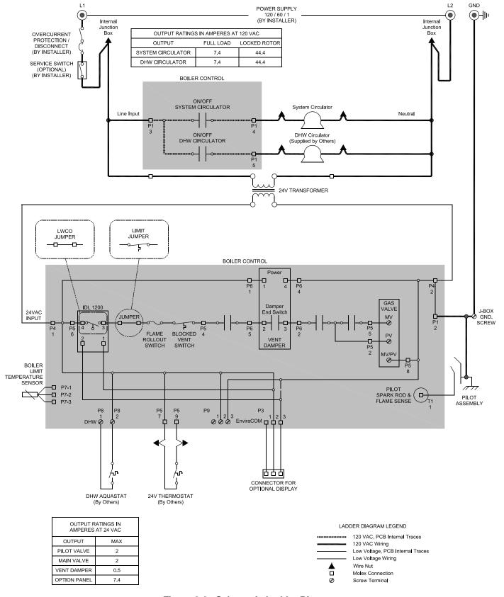
Figure 8-2: Schematic Ladder Diagram
