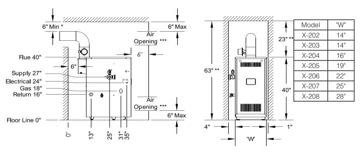
Figure 1-3: Minimum Closet Clearances
