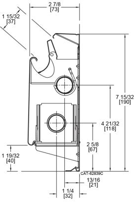
DIMENSIONS IN "[]" ARE SHOWN IN MILLIMETERS.
